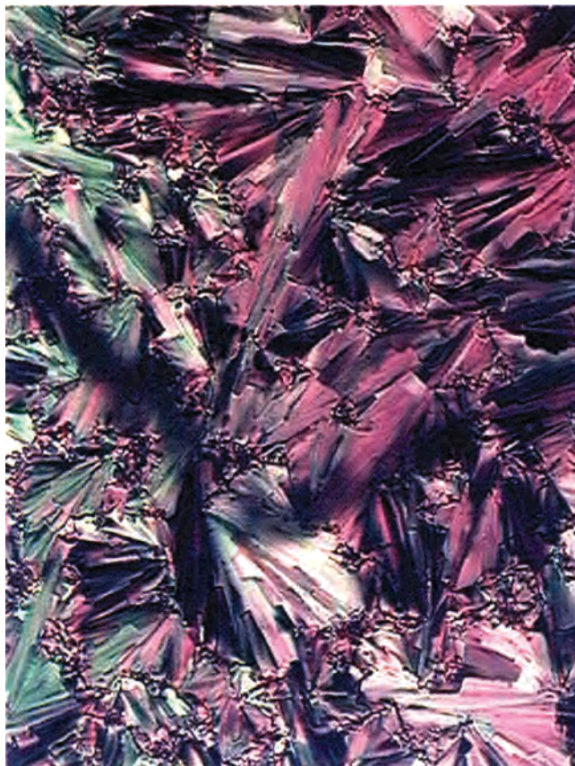
Figure 4. Polarized micrographs observed for the S_C phase of the binuclear 4.21 ( R^1 = OC_{12}H_{25} , R^2 = p-C_{14}H_{29}O-C_6H_4 ).
